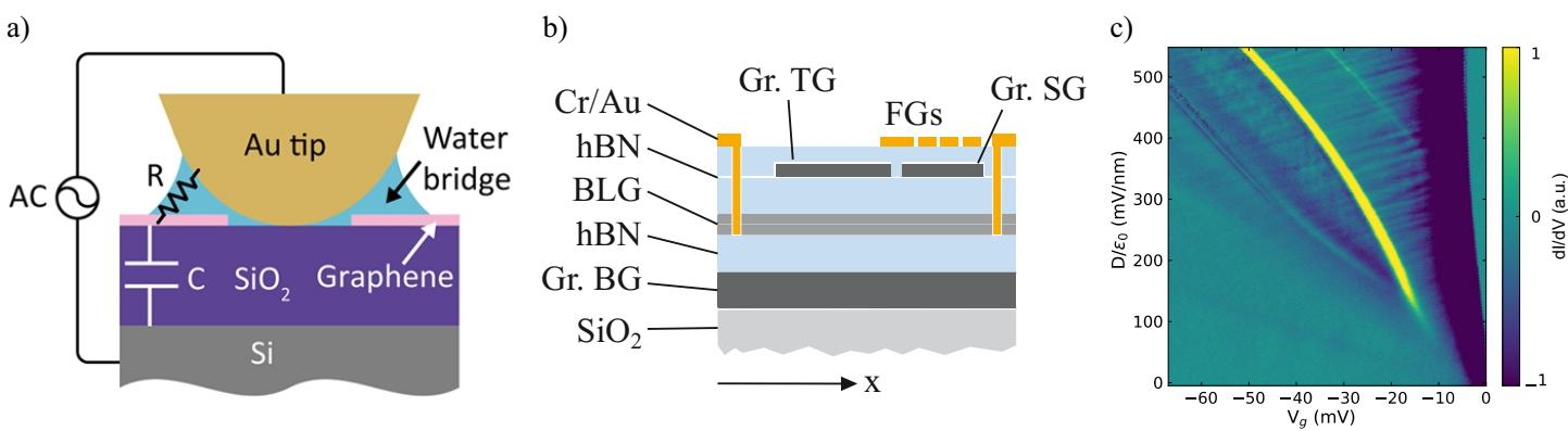
a) Schematic showing the working principle of EFLAO, using an AC-field between a sharp AFM tip and the substrate to oxidize the graphene below the tip. Taken from [3] b) Schematic sideview of the device. The Gr. TG allows to access and tune the magnetic phases and the Gr. SGs allow for the confinement of charge carriers in close proximity. c) Displacement field vs effective gate voltage phase diagram of BLG. Sharp increases and decreases in differential current indicate phase transitions.
